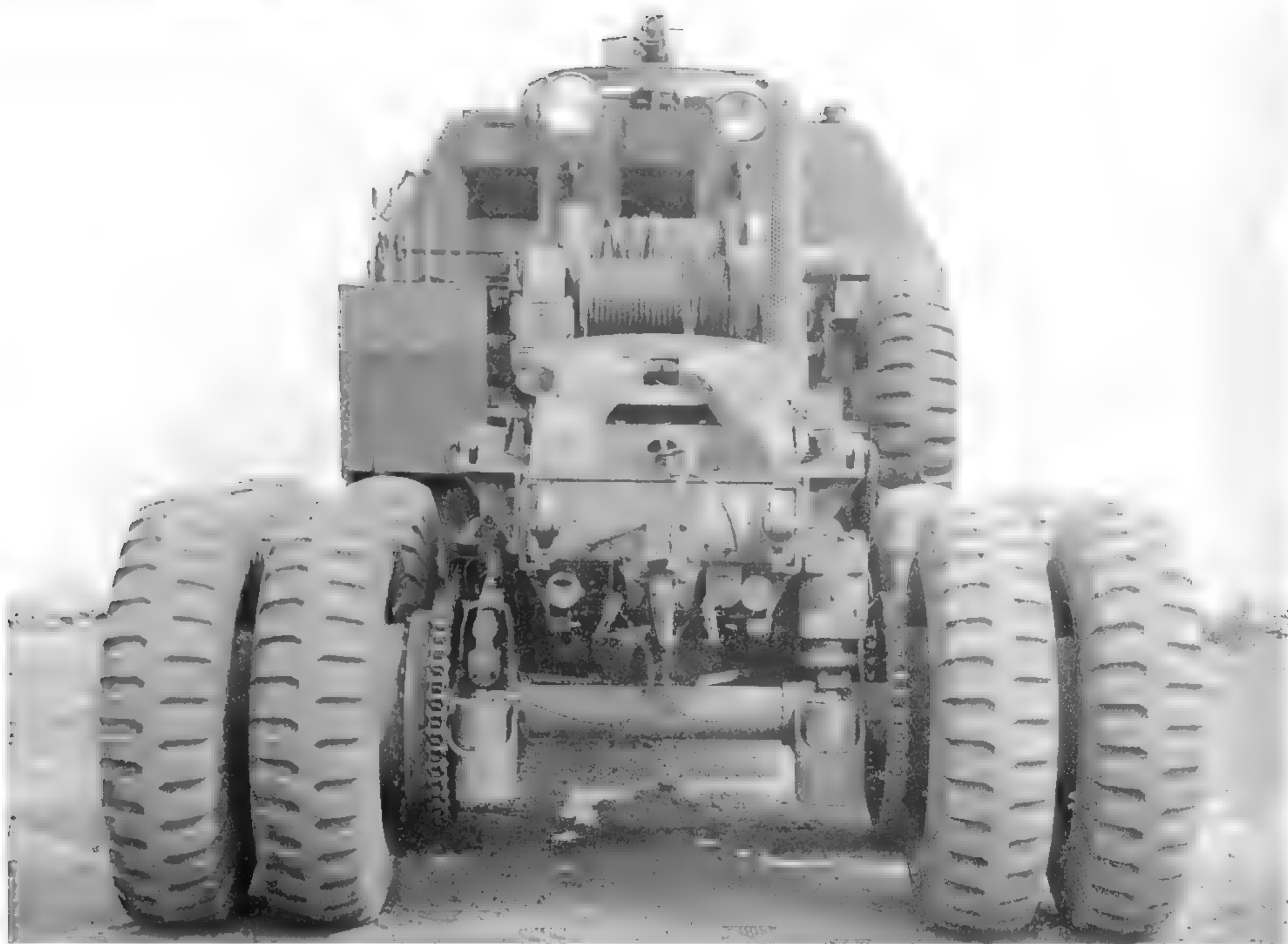
The pintle hook was relocated on the production vehicle, and was a more substantial design. The ring mount for the .50-caliber machine gun is just visible on the roof of the truck. (U.S. Army photo)
